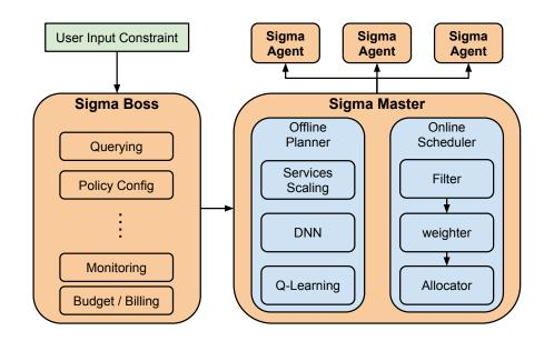
Figure 8.5. Sigma Architecture
