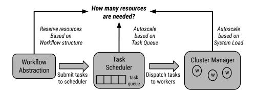
Figure 7.1: Resource Provisioning for HTC Workflows
