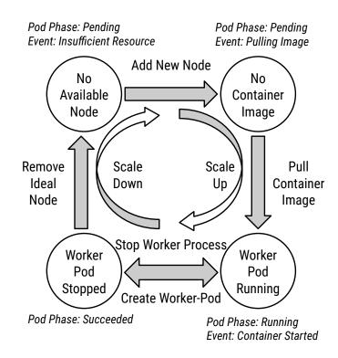
Figure 7.10: Lifecycle of a Worker-Pod
