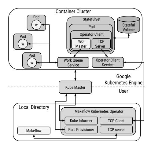
Figure 7.9: Makeflow Kubernetes Operator Architecture
