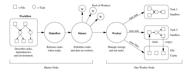
Figure 2.1: System Architecture Before Containers
