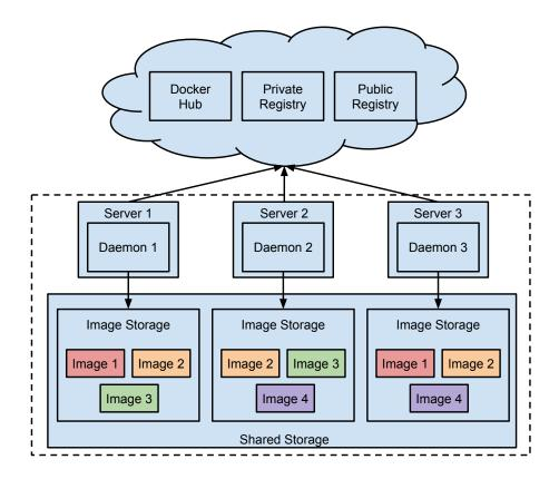
Figure 6.1. Docker on distributed storage, naive solution
