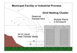
Figure 2 - GH Cluster schematic
