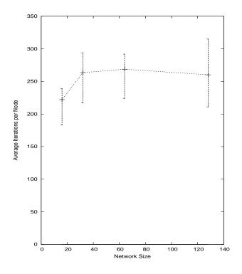
Fig. 6. The average number of iterations per node with error bars of five replications for optimization of DeJong's Sphere on a Patisserie network of 16, 32, 64, and 128 virtual nodes across 16 machines.
