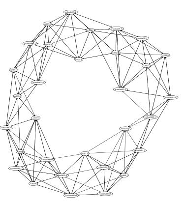
Fig. 1. Peer-to-peer network of sixteen machines each with two virtual nodes. Each node has seven PSO neighbors represented by directed edges with the topology defined by the Pastry network.
